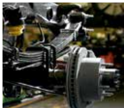
Asymmetrical rear suspension leaf springs.
